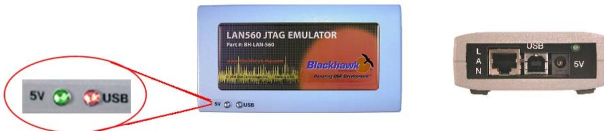
Figure 7 BH-LAN-560 Power LEDs
