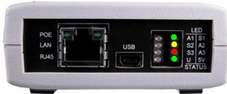
Figure 8- Bh560v2 End Panel LEDs (safe mode)
