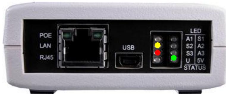
Figure 9 - Bh560v2 End Panel LEDs (normal mode)
