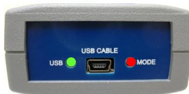
Figure 10 - USB560v2 End Panel LEDs (safe mode)
