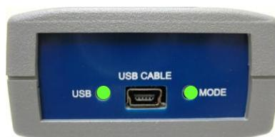
Figure 11 - USB560v2 Normal Operating Mode LED States<sup>1</sup>
