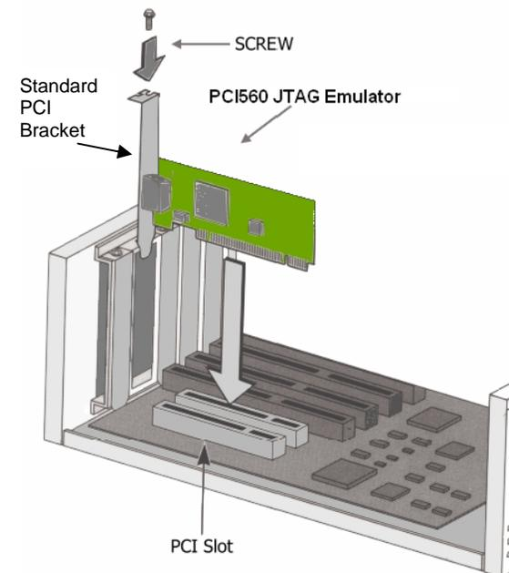
FIGURE 2 - **PCI560** Installation
